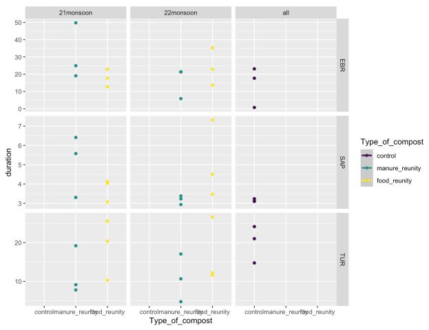
Figure 1. Infiltration time of the second inch of water in a single ring infiltrometer test by type of compost deployed in different years (columns; control plots were the same for both deployment years) at three sites in New Mexico (rows).
