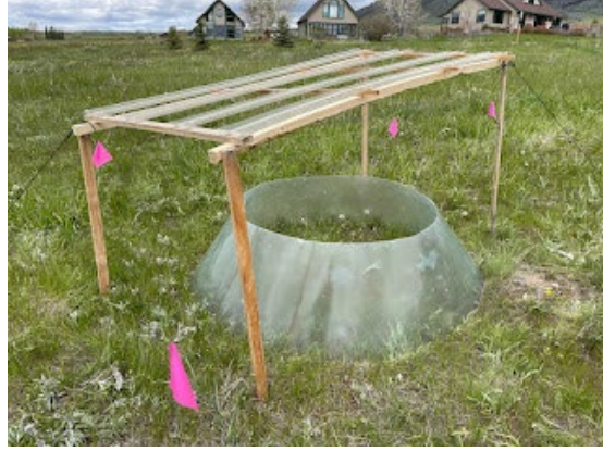
Figure 2. Photo of the open top chambers (OTCs) (on left) and open top chambers and rain out shelters (ROSs) (on right) for Objective 1.
