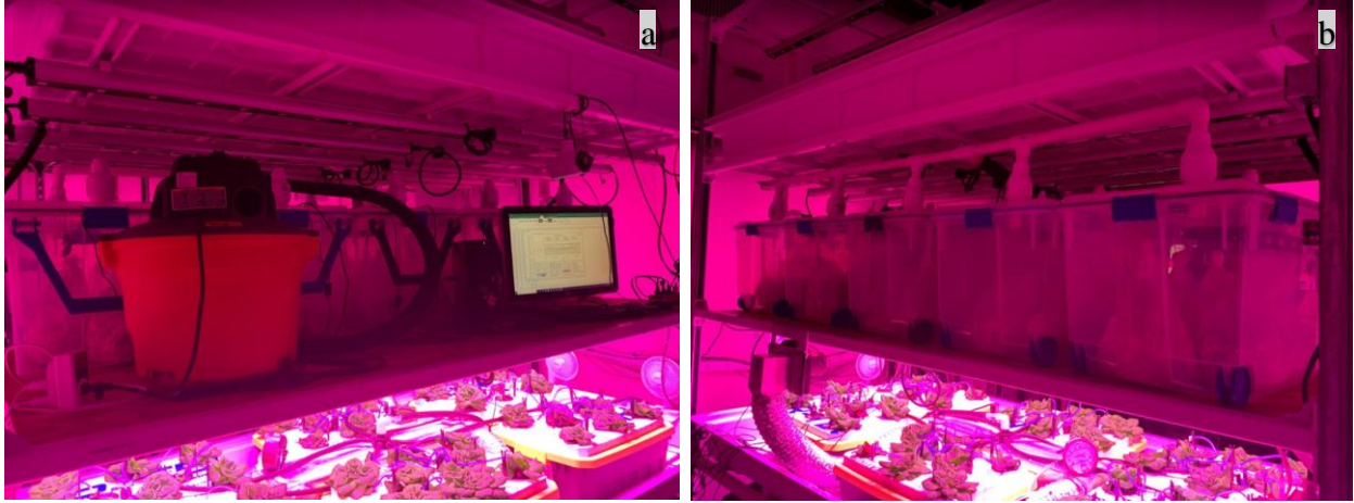
Figure 2: Photos showing the experimental units at the vertical farm facility at the University of Arizona's Controlled Environment Agriculture Center. Figure 3a shows the venting system and the data collection software Gaslab™. Figure 3b shows the manifold system for exhausting CO 2 .
