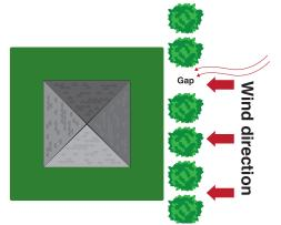
Figure 6. A gap in the windbreak accelerates wind-force to enter the protected area.
