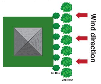
Figure 1. Windbreaks should be perpendicular to prevailing winds.
