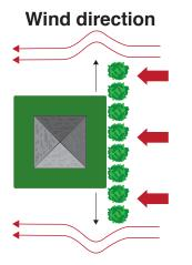
Figure 4. Windbreak extension reduces wind from whipping around the ends of the area to be protected.
