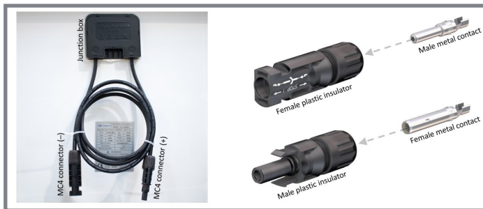
Figure 6. Junction box with a positive and negative lead on the back of a solar panel (left); and female and male configurations of an MC4 connector.
