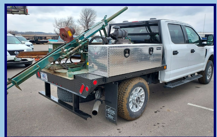
Soils truck rigged with flat bed and the old giddings.
