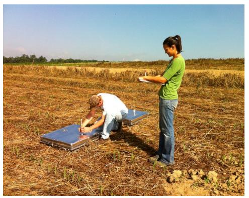
Samples collected with syringes and analyzed on the gas chromatograph
