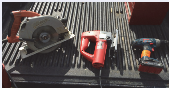
A circular saw, a jig saw, and a screw gun are the only power tools needed for the installation. Photo: Chris Lent, NCAT
