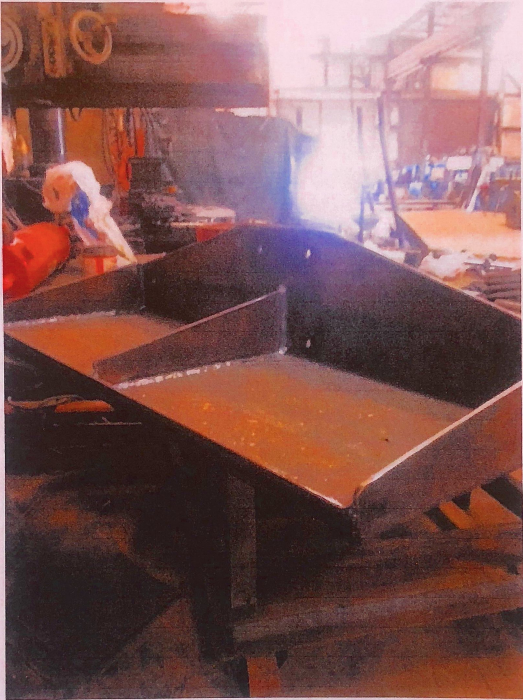
6. Engine, hydraulic pump, hydraulic fluid reservoir platform. Will be bolted to the distal end of the unit behind the axle.
