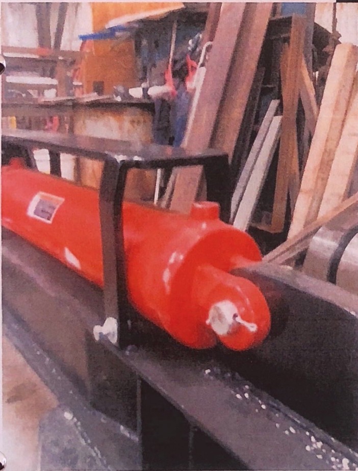
8. Distal End of hydraulic cylinder. Hydraulic cylinder covered by gate valve mounting plate for operation of cylinder and protection of hydraulic lines and cylinder.
