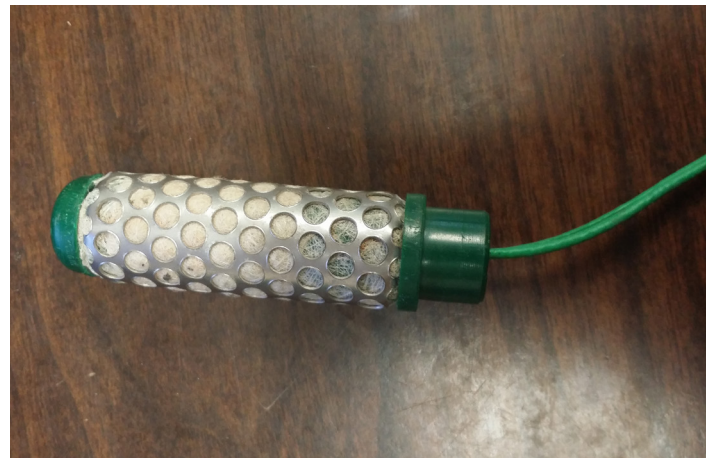
Fig. 2. The Irrrometer Watermark is an example of an electrical resistance block.
