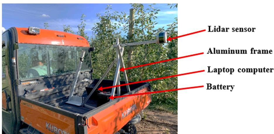
Fig. 3. Point cloud data acquisition system was driven by a utility vehicle.
