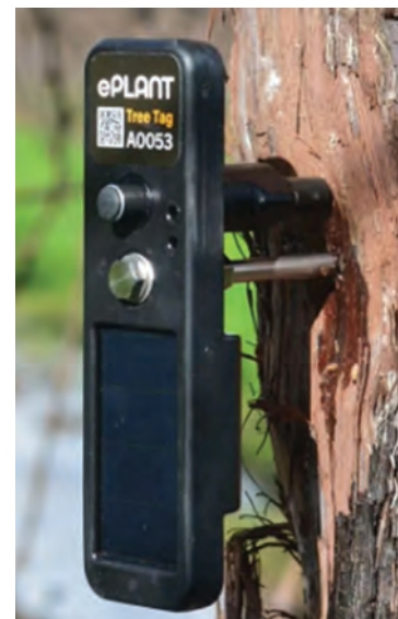
The ePlant measures plant growth and biomechanics.
