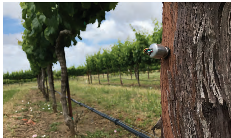
The FloraPulse Tensiometer attaches to the trunk of a grapevine for accurate water potential measurement of woody plants.
