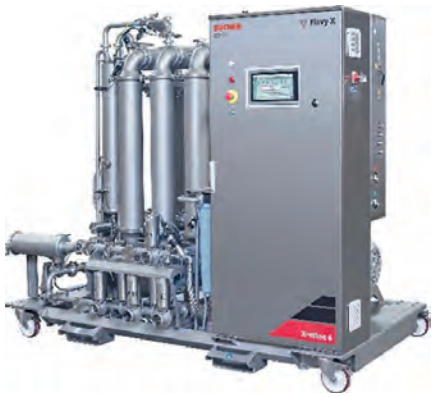
The Bucher Vaslin Flavy-X 6 module crossflow filter can include their energy saving module.
